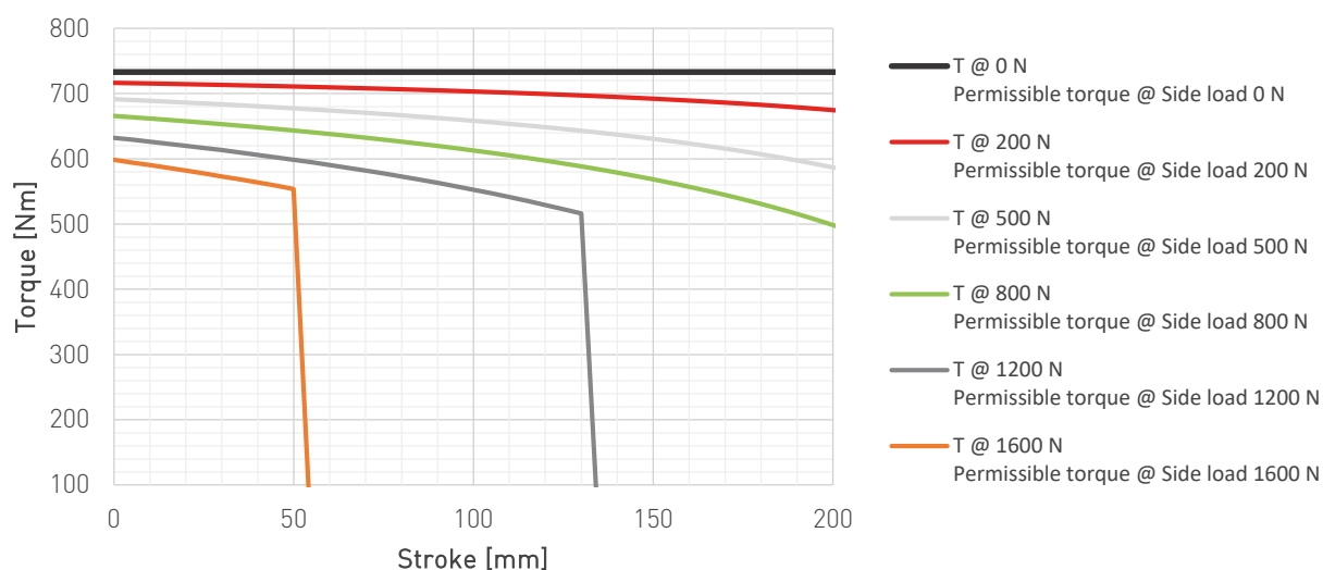
Permissible torque for a given side load EA200 - stroke 200 mm
