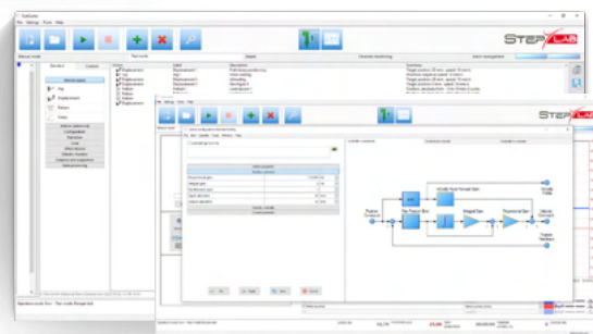
Multiaction module: test sequence definition by mean of several simple actions highly configurable
