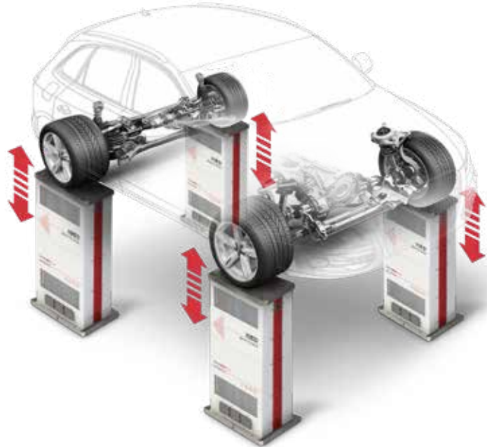
Damper Test System HUD20 with 4 synchronized machines
